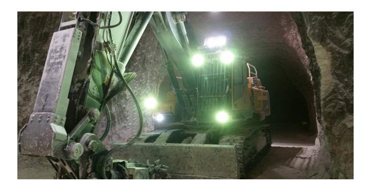
Placoplatre specializes in the extraction of gypsum in France. They use excavators specially equipped with a milling cutter, in a harsh and unforgiving underground environment. After fitting white LED lights the operators quickly found themselves in a cloud of white dust and visibility was drastically reduced causing issues with productivity and safety.
